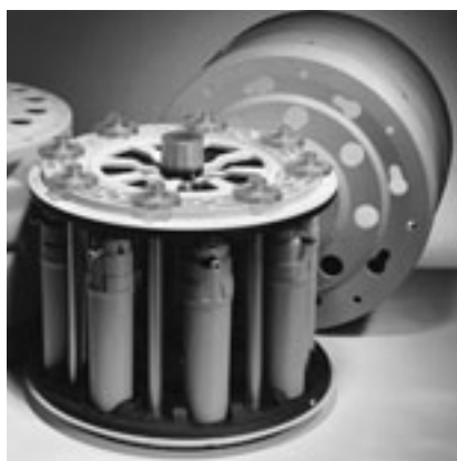
Using a multichambered reaction vessel, researchers can scale up microwave-assisted organic synthesis. (Reproduced with permission from Stadler, A.; et al. Org. Proc. Res. Dev. 2003, 7, 707–716.)
